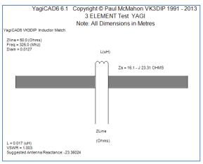
Figure 5 - Optimal L Match Physical
