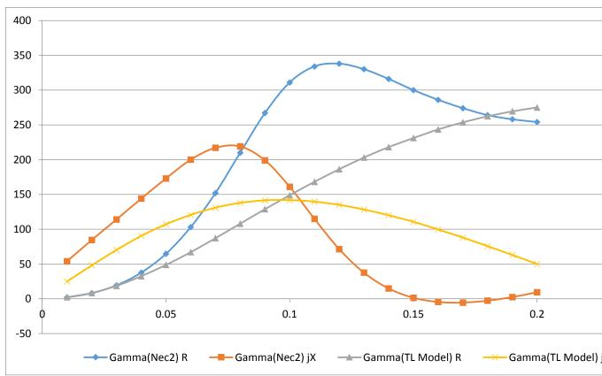
Figure 26 Graph of Gamma NEC2 results vs TL model predictions.
