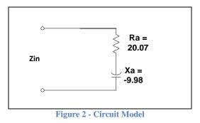
Here we see a dipole element (in this case a part of a three element Yagi array from Yagicad) which has an input impedance of 20.07 Ohms resistance ( $R_a$ ) in series with a negative or Capacitive reactance of 9.98 Ohms ( $X_a$ ). Mathematically we would write this as the complex impedance:
