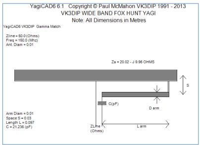
Figure 19 - YagiCAD calculated Gamma Match
