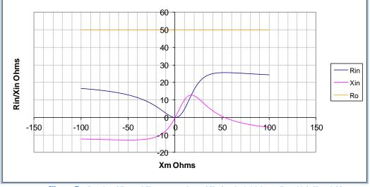
Figure 7 - Graphs of  $R_{\rm in}$  and  $X_{\rm in}$  versus values of  $X_{\rm m}$  for the initial case  $R_{\rm a}$  = 20.2,  $X_{\rm a}$ = -9.98
